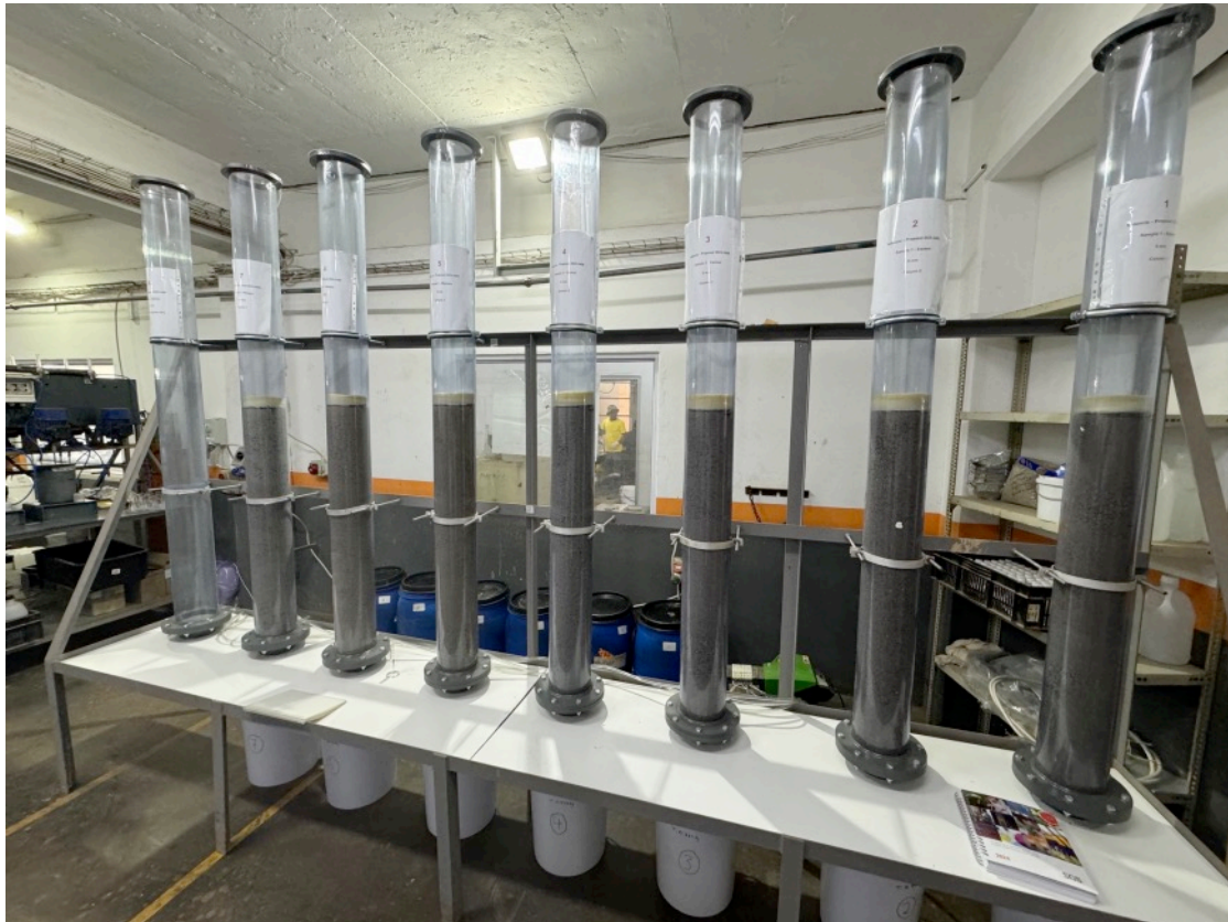
Figure 1: Leaching Columns at SGS South Africa
